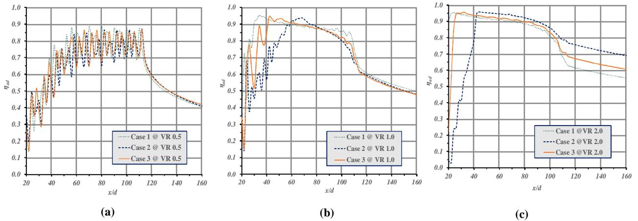
**Figure 5: Variation of laterally averaged film cooling effectiveness for Case 1, Case 2 and Case 3, with backward injection at (a) VR=0.5 (b) VR=1.0 (c) VR=2.0.**
