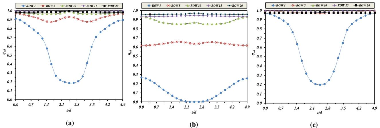
Figure 9. Lateral distribution of film cooling effectiveness with mix injection at velocity ratio  $VR=2.0$  for (a) case 1 (b) case 2 (c) case 3.
