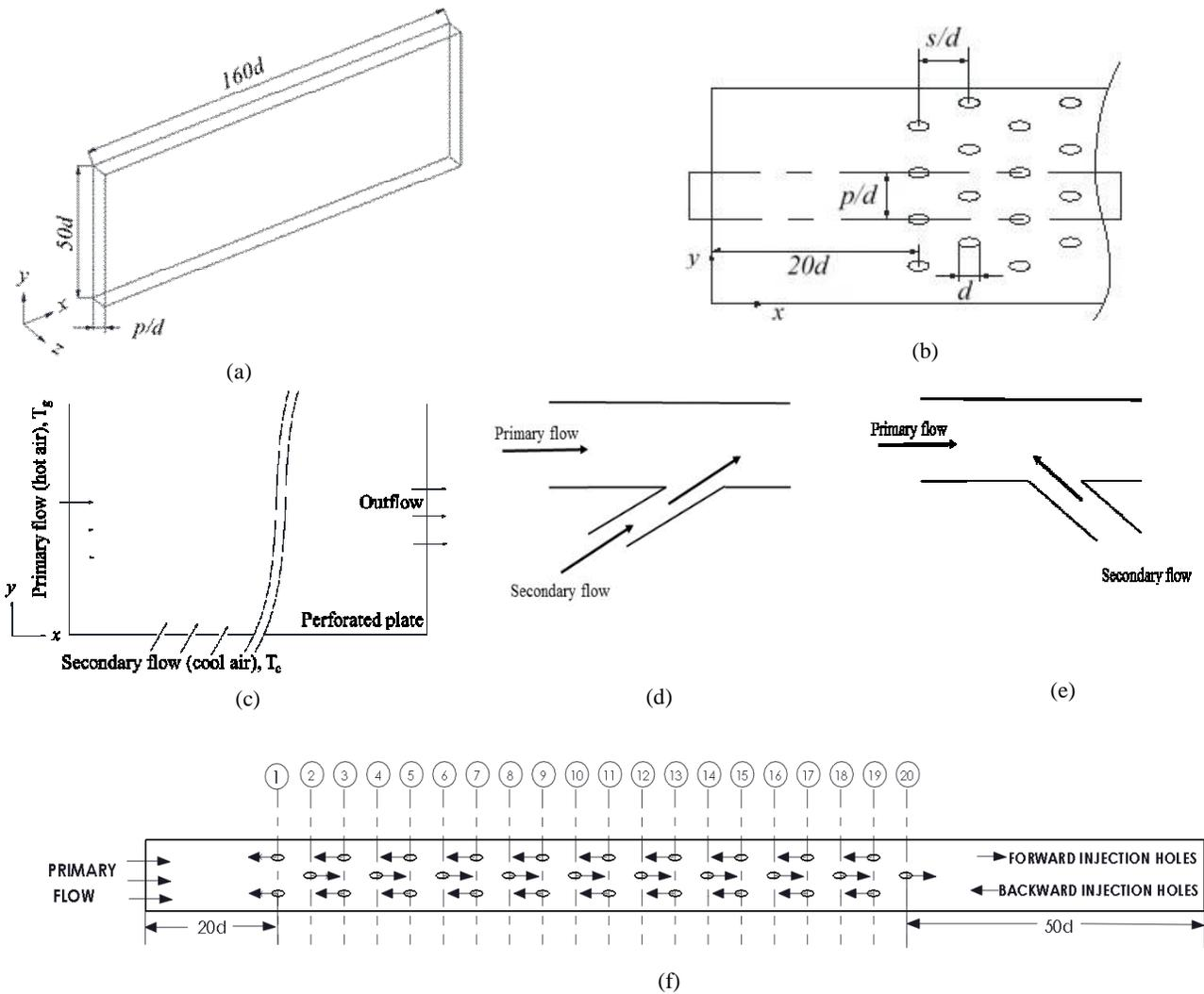
**Figure 1. (a) 3D computational domain (b) Details of holes arrangement on the wall [12] (c) Flow schematic (d) Forward injection (e) Backward injection and (f) Mix injection.**
