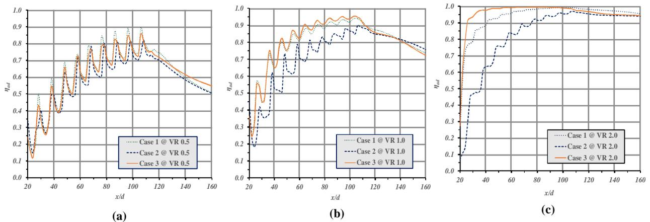
**Figure 6: Variation of laterally averaged film cooling effectiveness for Case 1, Case 2 and Case 3, with mix injection at (a) VR=0.5 (b) VR=1.0 (c) VR=2.0.**
