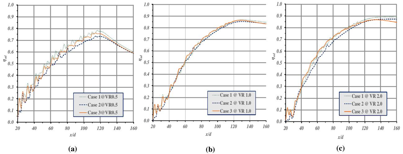
**Figure 4: Variation of laterally averaged film cooling effectiveness for Case 1, Case 2 and Case 3, with forward injection at (a) VR=0.5 (b) VR=1.0 (c) VR=2.0.**
