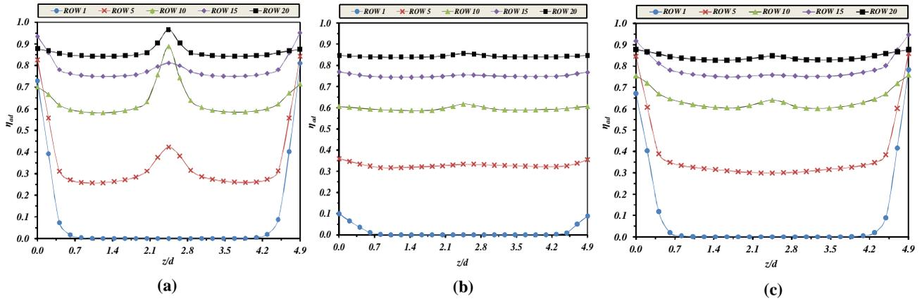
Figure 7. Lateral distribution of film cooling effectiveness with forward injection at velocity ratio  $VR=2.0$  for (a) case 1 (b) case 2 (c) case 3.
