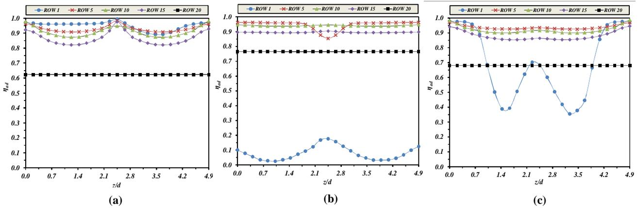
Figure 8. Lateral distribution of film cooling effectiveness with backward injection at velocity ratio  $VR=2.0$  for (a) case 1 (b) case 2 (c) case 3.
